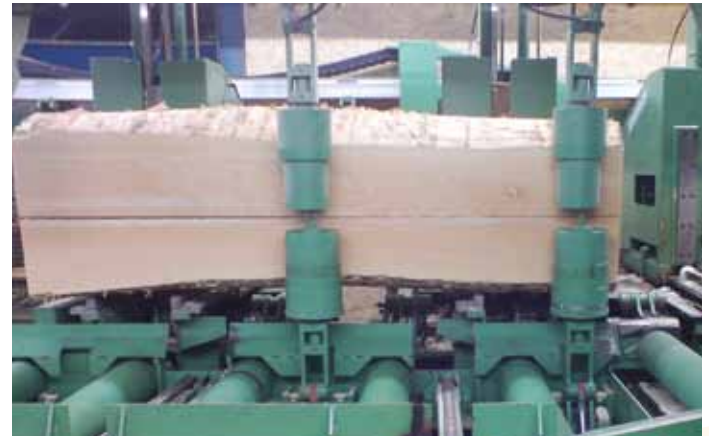
Circular saw with automatic singularization of both half boards
