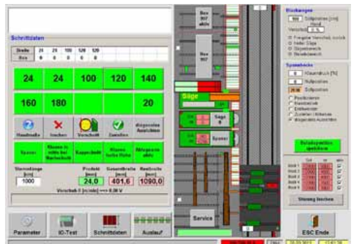
Automatic control of log carriage
